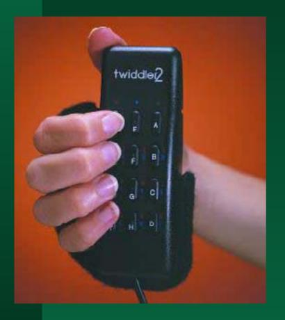
The Twiddler2 chorded keyboard is designed for onehanded input with an array of 12 finger keys and six thumb keys.
